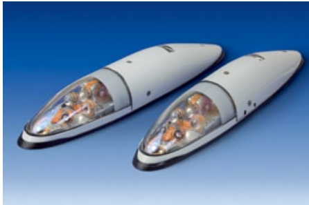
LED Navigation Lights 2LA002750-45 (NVIS red/IR) 2LA002750-46 (NVIS green/IR)
