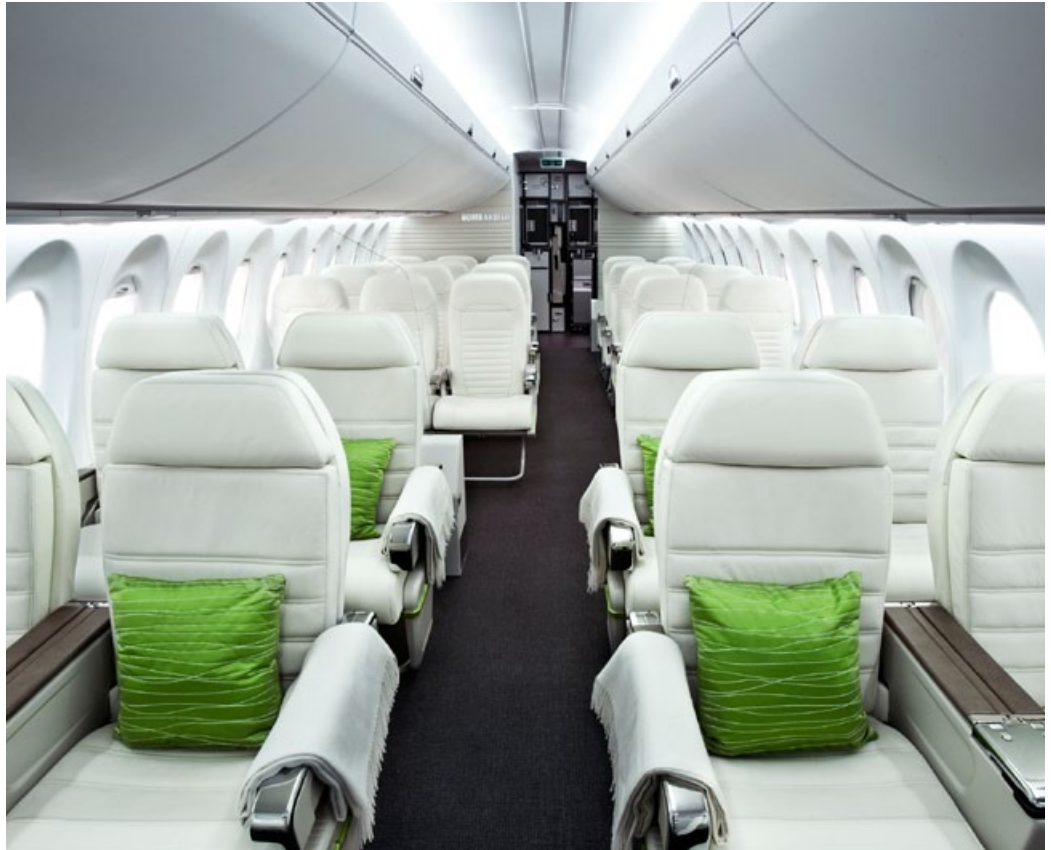
UTC Aerospace Systems wash light system 1005-01X-001 provides a homogeneous illumination that can be tuned from warm to cool white. This full LED ceiling and side wall lighting for cabins, galleys and lavatories will be standard on board the Bombardier CSeries* aircraft.
