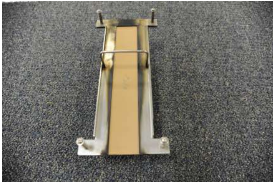
Figure 4. Alternate Spring-Loaded Test Sample Clamping
