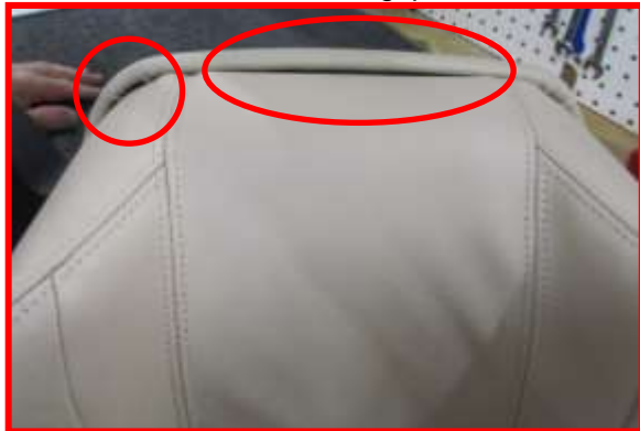
8.11 Unacceptable Condition Non uniform gaps
