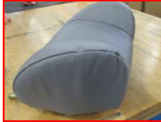
8.10 Unacceptable Condition Wings not fully filled out – loose leather
