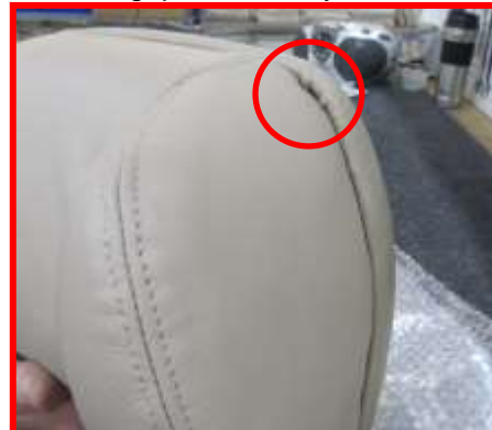
8.12 Unacceptable Condition Non uniform gaps created by leather bunching
